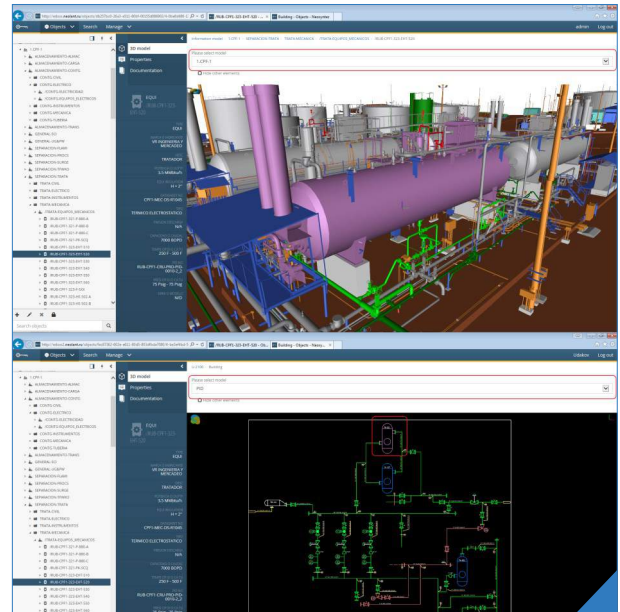
Accessing data of a tank through 3D models and P&ID
