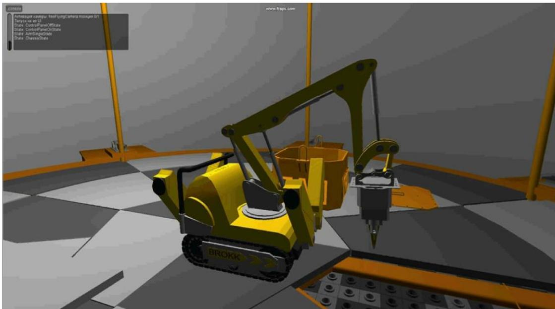
Figure 2. Simulation: dismantling radioactive graphite stack of a nuclear reactor
