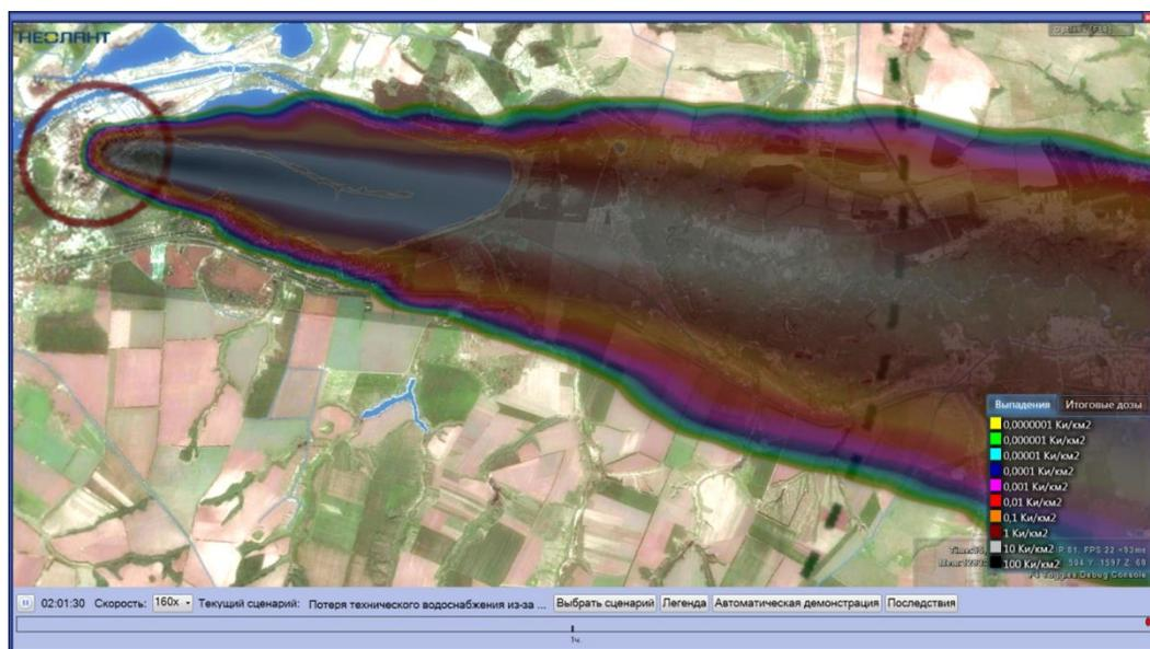
Figure 3. Visualization: Radioactive contamination spread simulation around a nuclear power plant
