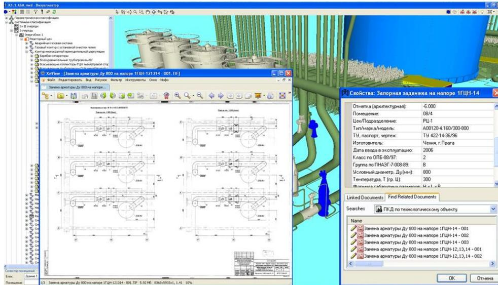
Figure 1. Access to plant data from the 3D model
