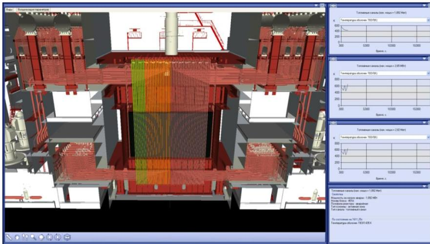
Figure 4. Simulated scenario: failure of a downflow pipe in a nuclear power unit
